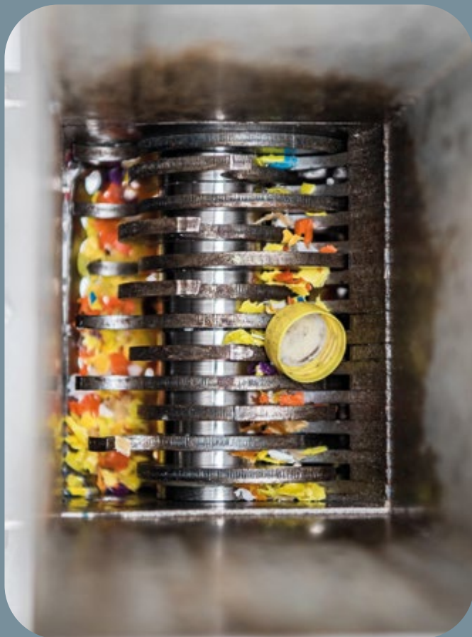
The shredder nicknamed the Tisza Crocodile, which was created using the designs of Precious Plastic. The machine can expertly handle hard plastic caps as well. Photo: Attila Molnár
